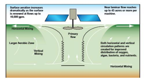
The SolarBee's high flow mixing action accelerates the normal purification process in the lake through gentle, thorough mixing and surface re-aeration.
